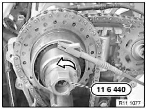
Attach special tool 11 6 440 to camshaft adjustment unit on cylinder bank 5 to 8 and move at 40 Nm to left-hand stop.
