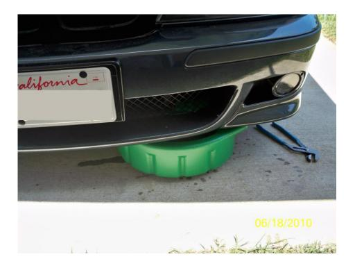
Remove belt tensioners. Remove terminal from alternator, and remove alternator. Keep drain pan under alternator, a lot of coolant will come out, (do not skip this step, you will get water in oil pan if you don't).
