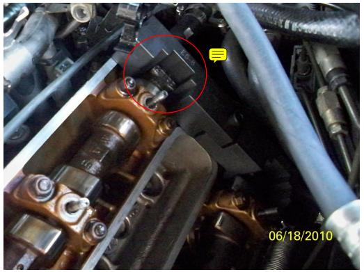
Tap on the top of the fixture blocks with the wooden handle of a hammer, or dead blow mallet to seat blocks against head surface.
