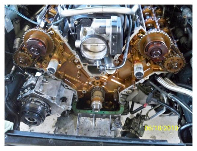
Cover oil pan area with rag, and use a razor to scrape and clean gasket surfaces.
