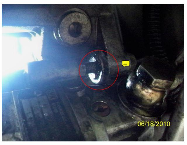
Drain the oil, and Remove lower oil pan. There are many bolts. I broke them loose with a ratchet, then used a drill with a socket to remove the rest. Check out pan for pieces of guides. Note: if yo find no pieces, it does not necessarily mean that the guides are good. This engine had 78k miles on it, and the guides appeared to be good with no parts in the pan. But, when I pulled off the chain, pieces of the guides were falling off. The chain was holding the pieces of the guides in place!
