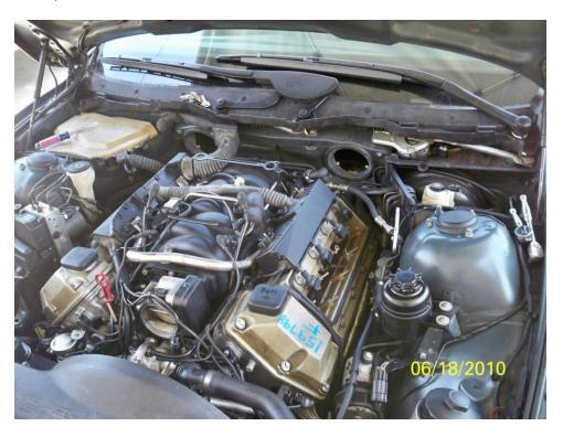
Unplug engine wiring harness from engine.
