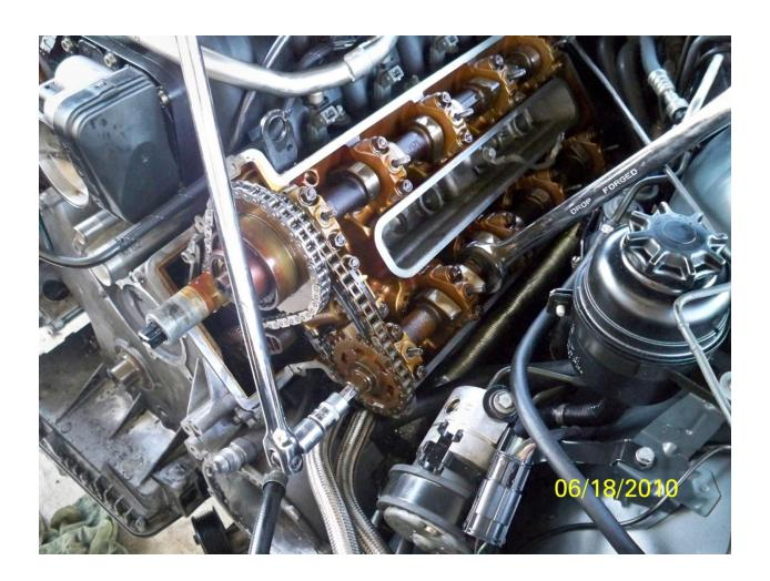
On the rear of each camshaft there is a machined square. 2 sides are precision ground, and 2 sides are left as cast. One of the cast sides have numbers stamped into them. After loosening all 4 cam bolts, use wrench to rotate cams until the side with the stampings are facing up away from the face of the head. Once again, If you turn the cam, and the cam stops, turn the cam the opposite direction, as a valve must be contacting a piston. You can bend a valve if you put too much force on it.
