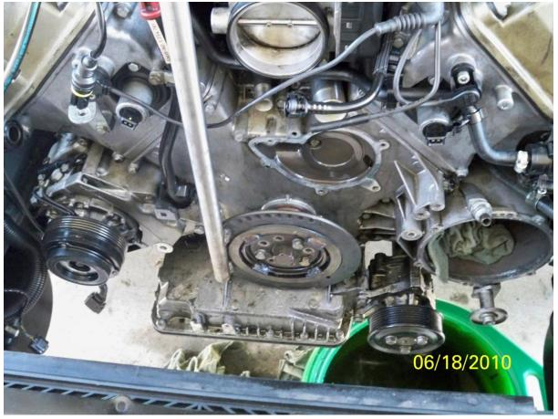
Remove special tool, but leave bolt in crank for now.
