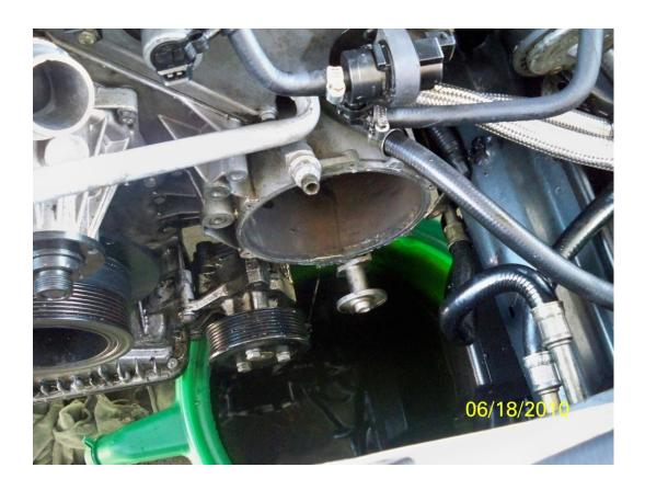
Remove radiator, Egr pipe, and water pump. Remove crank pulley. Bolt special tool onto crank hub with a minimum of 3 bolts. Place a piece of wood in between passenger side of frame, and handle of special tool. Use large breaker bar and 1 1/16 socket to loosen crank bolt. The bolt is very tight, (300 ft pounds of torque). I used a ¾ breaker bar and socket, as I broke the ½ bar.
