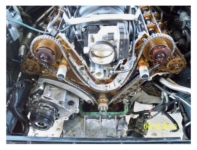
Wipe clean gasket surfaces, and apply silicone to oil pan gasket area (note green gasket on above photo). put steel coated gaskets in place, on water pump area and sides of timing cover. Place a small dab of silicone in corner of oil pan and block. Install lower timing cover. Be sure to remember to put bolts in bottom of cover through oil pan opening back.
