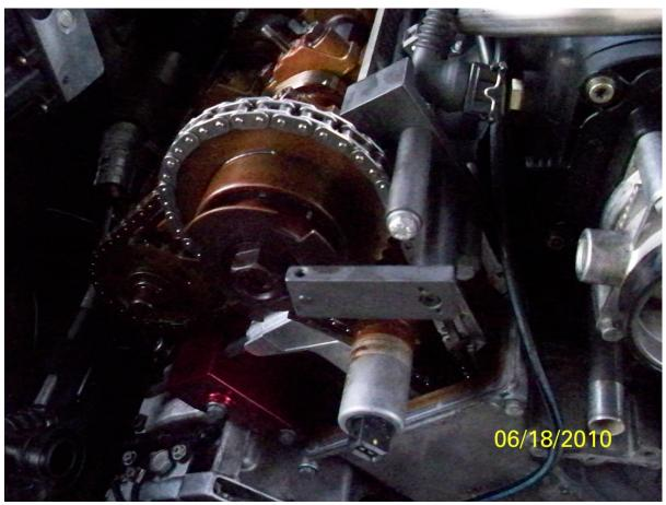
Remove tensioner block, and cam sensor disk fixtures.
