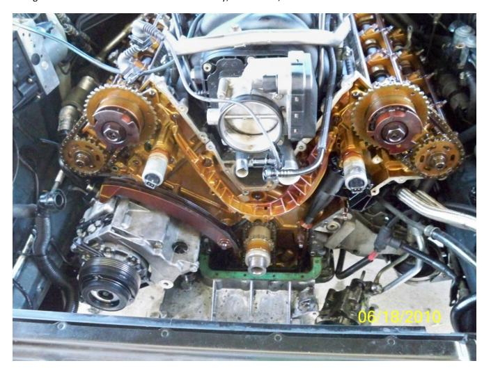
Remove timing chain guides, starting with tensioner side, then deflection rail. Remove last guide, and finally chain.
